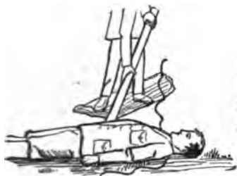
Prying off wire or rail with dry wooden bar. Stand on a dry board.
